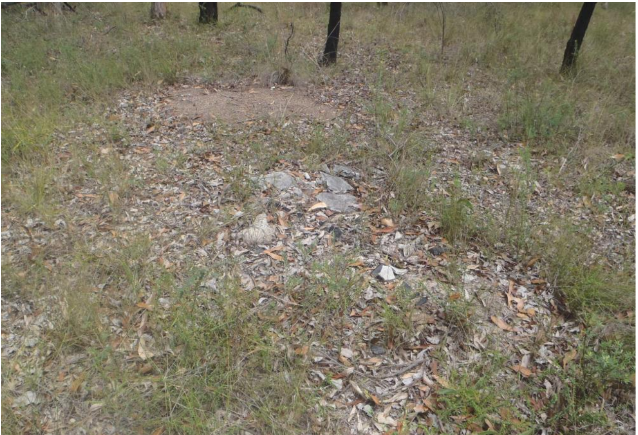
Photograph 11: Fragments of possible asbestos containing material
